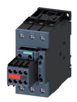
Power contactor, AC-3 65 A, 30 kW / 400 V 2 NO + 2 NC, AC / DC 20-33 V, with varistor 3-pole, size S2 screw terminals Perm. mounted auxiliary switch
