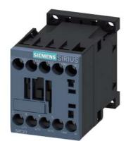
Power contactor, AC-3 7 A, 3 kW / 400 V 1 NO, 24 V AC, 50 / 60 Hz 3-pole, Size S00 screw terminal
