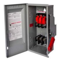
Siemens Low Voltage Circuit Protection Heavy Duty Safety Switch. 3-Pole 3-Wire Fused in a type 3R enclosure (outdoor). Rated 600VAC (200A). Special features: photovoltaic rated, positive ground, 10000 AIC disconnect.
