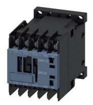
Power contactor, AC-3 16 A, 7.5 kW / 400 V 1 NO, 400 V AC, 50 Hz 400-440 V, 60Hz, 3-pole Size S00 ring cable lug connection
