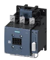
power contactor, AC-3 300 A, 160 kW / 400 V, AC (50-60 Hz) / DC operation 200-277 V AC/DC auxiliary contacts 1 NO + 1 NC 3-pole, frame size S10 busbar connections drive: electronic with PLC / SIMOCODE - interface and remaining lifetime signal
