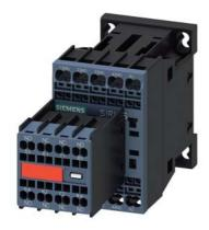
Contactor relay, 6 NO + 2 NC, 110 V AC 50 Hz / 120 V 60 Hz, Size S00, spring-type terminal, Captive auxiliary switch,
