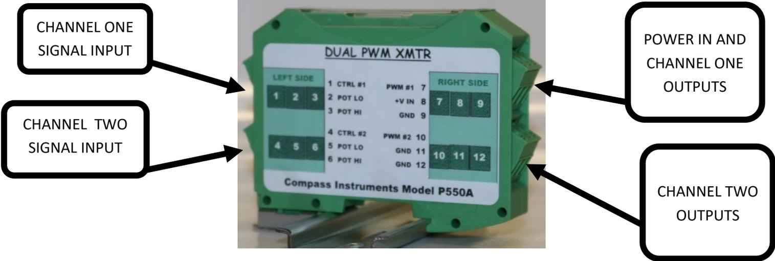
The Compass Instruments P550A Dual PWM Transmitter is a dual voltage to pulse width modulator. Each channel of the transmitter may be driven with a variable 0 to 5VDC signal to produce a proportional pulse width modulated output capable of directly controlling devices requiring up to 5 amps of current. Each output operates at 488 Hz and can sink up to 5 amps of current and switch up to 30 volts DC. The input circuits are also designed to accommodate a 10K ohm potentiometer.
