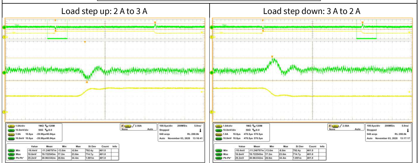
Figure 19 Transient response at 1 A step load current: I_o = 2\text{ A} - 3\text{ A} , (Ch1: I_o , Ch4: V_o ), pk-pk: 30.96 mV, fsw = 1000 kHz
