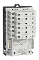
Electrically held lighting contactor, (convertible to mech. held), Amp rating 30A (tungsten 20A), 4 N.C. / 6 N.O. poles, 575-600V 60Hz/550V 50Hz coil, Non-combination type, Enclosure NEMA type (open), No enclosure
