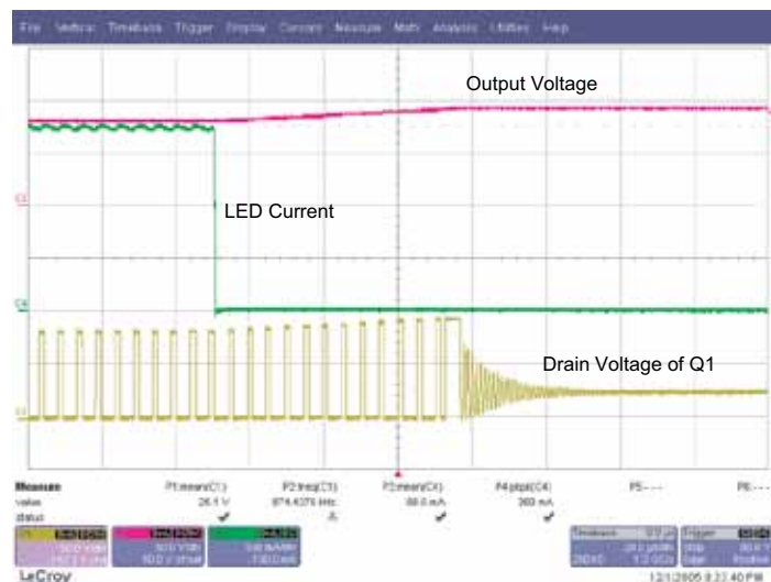
Fig. 6: Open LED Protection (20µs/div)
