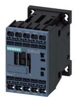
Contactor relay, 4 NO, 42 V AC, 50 / 60 Hz, Size S00, Spring-type terminal
