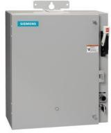
Pump control panel, Size 1, Three phase full voltage, Solid-state overload relay, OLR amp range 0.75-3.4A, 110V 50Hz / 120V 60Hz coil, Standard type contactor, 3A circuit breaker, HOA Sel Sw. <(>&<)> Start P.B., Enclosure NEMA type 3/3R, Weather proof outdoor use
