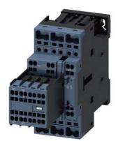
power contactor, AC-3 9 A, 4 kW / 400 V 2 NO + 2 NC, 220 V AC 50 / 60 Hz, 3-pole Size S0, Spring-type terminal Removable auxiliary switch
