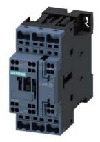
Power contactor, AC-3 38 A, 18.5 kW / 400 V 1 NO + 1 NC AC (50 - 60 Hz) / DC 200-280 V AC / DC, 3-pole Size S0, Spring-type terminals
