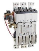
Mechanically held lighting contactor, Contactor amp rating 400A, 0 N.C. / 3 N.O. poles, 208VAC 60HZ coil, Non-combination type, Enclosure NEMA type (open), No enclosure
