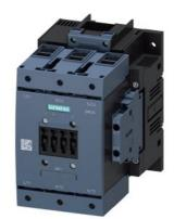
power contactor, AC-3 115 A, 55 kW / 400 V AC (50-60 Hz) / DC operation 380-420 V AC/DC auxiliary contacts 2 NO + 2 NC 3-pole, frame size S6 with box terminals drive: conventional screw terminal
