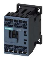
Coupling relay, AC-3 12 A, 5.5 kW / 400 V 1 NO, 24 V DC 0.85-1.85\* Us, with suppressor diode integrated Size S00, spring-loaded terminal
