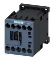
power contactor, AC-3 12 A, 5.5 kW / 400 V 1 NO, 24 V DC with diode integrated, 3-pole Size S00, screw terminal
