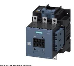
Traction contactor, AC-3 115 A, 55 kW / 400 V Coil 24 V DC x (0.7-1.25) PLC input 24-110 V DC Auxiliary contacts 2 NO + 2 NC 3-pole size S6 Busbar connections Coil connection: Spring-type terminal
