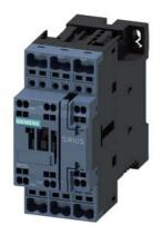
power contactor, AC-3 9 A, 4 kW / 400 V 1 NO + 1 NC, AC (50-60 Hz) DC operation 21-28 V AC/DC, 3-pole, Size S0, Spring-type terminal
