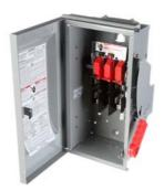
Siemens Low Voltage Circuit Protection Heavy Duty Safety Switches. Type: ENCLOSED, SAFETY SWITCH Std: CSA V. Rating: 240V A. Rating: 30 A Wattage: 3W No. Of Poles: 2P F. Rating: 60Hz Action: SINGLE THROW Material: 304SS Enclosure: TYPE 3R. 2-3 point mounting holes. O. Cycles: 10000 O. Temperature: (-20F-120F) AMBIENT TEMPERATURE Environmental Conditions: OUTDOOR
