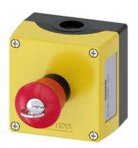
Enclosure for command devices, 22 mm, round, Enclosure material plastic, Enclosure top part yellow, 1 control point plastic, Control point in center, A=EMERGENCY STOP mushroom pushbutton red, 40 mm, with RONIS lock SB30, key-operated release, 1 NC, 1NO, screw terminal, floor mounting, 1xM20 each on top and bottom
