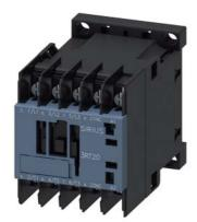
Power contactor, AC-3 7 A, 3 kW / 400 V 1 NC, 100 V AC, 50 Hz 100-110 V, 60 Hz, 3-pole, Size S00, ring cable lug connection
