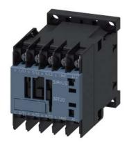
Power contactor, AC-3 16 A, 7.5 kW / 400 V 1 NO, 24 V DC 3-pole, Size S00 ring cable lug connection
