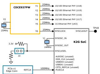
Figure 22. Clock Inputs
