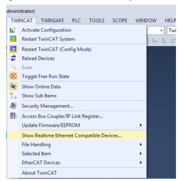
5. Select the Ethernet port from the list of compatible devices, and press Install. This installs a Beckhoff EtherCAT driver. When installed, the Ethernet port appears in Installed and ready to use devices, as shown in Figure 10.
