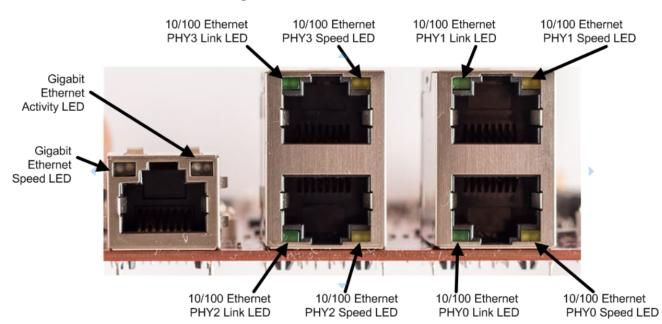
Figure 35. Ethernet LED Positions
