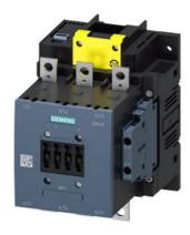
Power contactor, AC-3 115 A, 55 kW / 400 V Coil AC 50/60 Hz and DC 200-277 V x (0.8-1.1) F-PLC input 24 V DC 3-pole size S6 Auxiliary contacts 2 NO + 2 NC Main circuit: Busbar Control and auxiliary circuit: screw terminal
