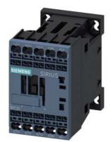
power contactor, AC-3 12 A, 5.5 kW / 400 V 1 NC, 24 V DC 0.85-1.85\* US, with Suppressor diode integrated Size S00, Spring-type terminal
