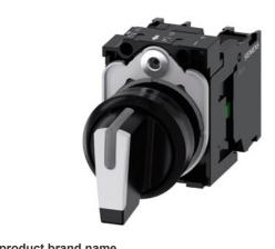
Selector switch, illuminable, 22 mm, round, plastic, white, selector switch, short, 3 switch positions I-O-II, latching, 10:30h/12h/13:30h, with holder, 1 NO, 1 NO, screw terminal, with laser labeling, upper case and lower case, always upper case at beginning of line
