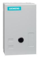
Electrically held lighting contactor, Contactor amp rating 30A, 0 N.C. / 3 N.O. Poles, 277VAC 60HZ coil, Non-combination type, (no disconnect device), Enclosure NEMA type 1, Indoor general purpose use
