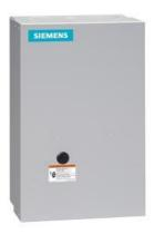
Electrically held lighting contactor, Contactor amp rating 30A, 0 N.C. / 6 N.O. Poles, 220VAC 50HZ/240VAC 60HZ coil, Non-combination type, (no disconnect device), Enclosure NEMA type 1, Indoor general purpose use
