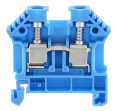
Feed-through terminal, Screw connection, Mounting type: Mounting rail TS 35/7.5, Rated cross-section: 10 mm<sup>2</sup>, Width: 8 mm, Colour: Blue
