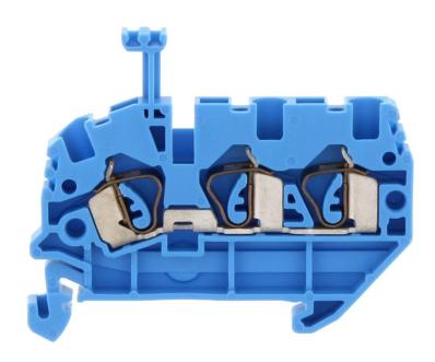
Ex feed-through terminal ATEX-certified, Tension-spring connection, Mounting type: Mounting rail TS 35/7.5, Rated cross-section: 2.5 mm², Width: 5.1 mm, Colour: Blue
