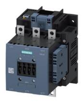
power contactor, AC-3 150 A, 75 kW / 400 V AC (50-60 Hz) / DC operation 200-277 V AC/DC auxiliary contacts 2 NO + 2 NC 3-pole, frame size S6 busbar connections drive: electronic with PLC interface 24 V DC spring-loaded terminal
