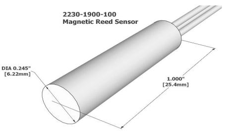
All measurements are in Inches [millimeters]
