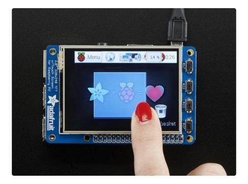
Is this not the cutest little display for the Raspberry Pi? It features a 2.8" display with 320x240 16-bit color pixels and a resistive touch overlay. The plate uses the high speed SPI interface on the Pi and can use the mini display as a console, X window port, displaying images or video etc. Best of all it plugs right in on top!
