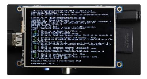
One fun thing you can do with the display is have it as your main console instead of the HDMI/TV output. Even though it is small, with a good font you can get 20 x 40 of text. For more details, check out https://github.com/notro/fbtft/wiki/Boot-console ()
