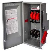
Siemens Low Voltage Circuit Protection Heavy Duty Safety Switches. Type: ENCLOSED, SAFETY SWITCH Std: UL V. Rating: 600V A. Rating: 30 A No. Of Poles: 3P F. Rating: 60Hz Action: SINGLE THROW Material: STEEL Enclosure: TYPE 1. 2-3 point mounting holes. O. Cycles: 10000 O. Temperature: (-20F-120F) AMBIENT TEMPERATURE Environmental Conditions: INDOOR
