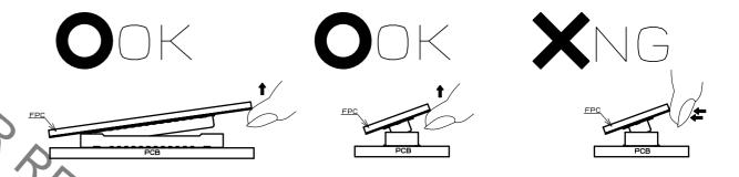
FPC IS NOT RIGID. THE CONNECTOR CAN BE BROKEN. PLEASE CHECK THE ACTION OF THE FPC TO BE USED REPEATEDLY AT THE TIME OF TRIAL PRODUCTION. BE CAREFUL TO UN-MATE THEM FROM THE PITCH DIRECTION. THE CORNER CAN ALSO RISK TO PUTTING STRESS ON CONTACTS.
