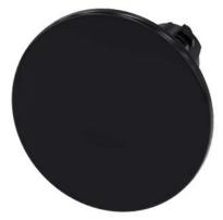
Mushroom pushbutton, 22 mm, round, plastic, black, 60 mm, latching, Pullto-unlatch mechanism
