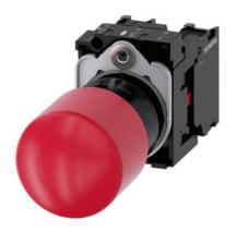
EMERGENCY STOP mushroom pushbutton, 22 mm, round, plastic, red, 30 mm, positive latching, according to EN ISO 13850, rotate-to-unlatch, without yellow backing plate, with holder, 1 NC, 1 NC, screw terminal
