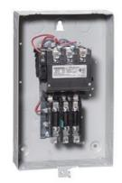
Non-reversing motor starter, Size 2 1/2, Single phase, 2-pole, Amb compensate bimetal OLrelay Contactor amp rating 60Amp 190 220/220 240V 50/60HZ coil, Non-combination type, Enclosure type 1, Indoor general purpose use
