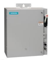
Pump control panel, Size 1, Three phase full voltage, Solid-state overload relay, OLR amp range 3-12A, 380-440/440-480V 50/60Hz coil, Standard type contactor, 10A circuit breaker, HOA Sel Sw. <(>&<)> Start P.B., Enclosure NEMA type 3/3R, Weather proof outdoor use
