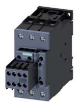
Power contactor, AC-3 80 A, 37 kW / 400 V 2 NO + 2 NC, 400 V AC, 50 Hz 400-440 V, 60 Hz 3-pole, size S2 screw terminals
