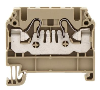
Feed-through terminal, Push-in connection, Mounting type: Mounting rail TS 35/7.5, Rated cross-section: 4 mm², Width: 6.1 mm, Colour: Beige
