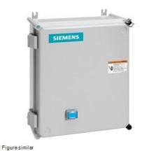
Reversing motor starter, Size 2 1/2, Three phase full voltage, Amb. compensate bimetal OLR, Contactor amp rating 60A, 208VAC 60Hz coil, Non-combination type, Enclosure type 4X fiberglass, Water/dust tight noncorrosive
