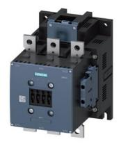
Traction contactor, AC-3 225 A, 110 kW / 400 V Coil 24 V DC x (0.7-1.25) PLC input 24-110 V DC Auxiliary contacts 2 NO + 2 NC 3-pole size S10 Busbar connections Coil connection: screw terminal
