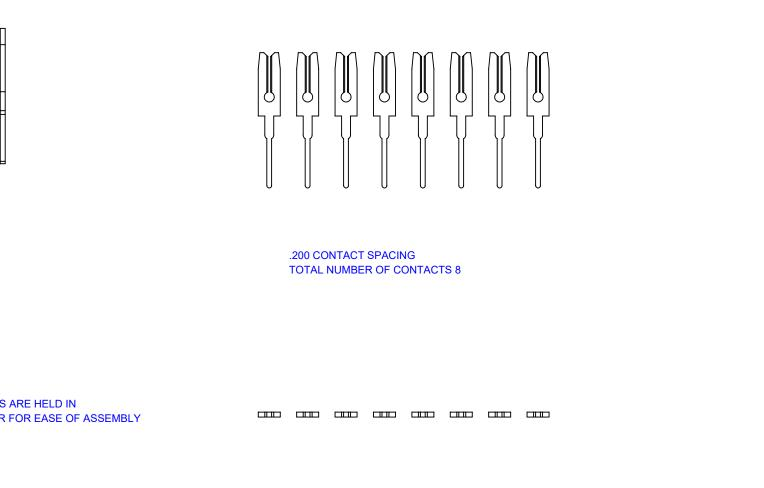
ACAD REFERENCE NO.: 103 Assembly **103 SERIES - HORIZONTAL CONTACT PATTERN** DRAWN: C.B DATE: April 8, 2020 CHECKED: DATE: THESE DRAWINGS AND SPECIFICATIONS SCALE: 2:1 SHEET 1 OF 1 EDAC INC ARE THE PROPERTY OF EDAC INC. AND TORONTO, ONTARIO SHALL NOT BE REPRODUCED, OR COPIED 103 Assembly ISSUE DRAWING NUMBER: OR USED AS THE BASIS FOR THE CANADA MANUFACTURE OR SALE OF APPARATUS 1 YOUR CONNECTION TO QUALITY & SERVICE PART NUMBER: 103-008-251-200 WITHOUT WRITTEN PERMISSION.
