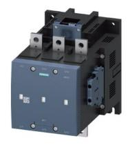
vacuum contactor, AC-3 500 A, 250 kW / 400 V AC (50-60 Hz) / DC operation 96-127 V AC/DC auxiliary contacts 2 NO + 2 NC 3-pole, frame size S12 busbar connections drive: electronic with SPS interface DV 24 V
