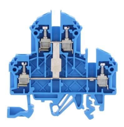
Double-level terminal, Screw connection, Mounting type:Mounting rail TS 35/7.5 and TS 32, Rated cross-section: 2.5 mm², Width: 5 mm, Colour: Blue
