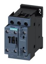
power contactor, AC-3 9 A, 4 kW / 400 V 1 NO + 1 NC, 208 V AC, 50 / 60 Hz, 3-pole, Size S0, screw terminal
