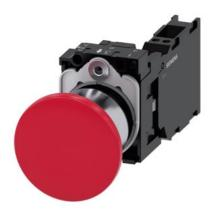
Mushroom pushbutton, 22 mm, round, metal, shiny, red, 40mm, latching, pull-to-unlatch mechanism, with holder, 1 NO+1 NC, spring-type terminal, with laser labeling, upper case
